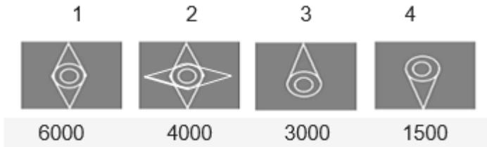
Harmonic images at 6000 and 4000 rpm are not a single still image, but double and quadruple. Single image appears at 3000 and 1500 rpm. 1500 is half of 3000 and the same single image appears, therefore, the actual speed of the object is 3000 rpm.
